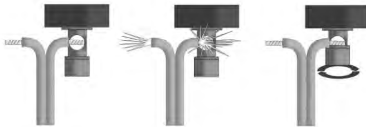
Do not allow strands to cause a short
