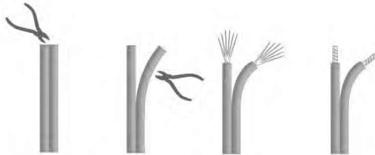
Properly twist wire to eliminate stray strands
